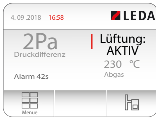
Fig. 7.3 Display in the event of a fault
